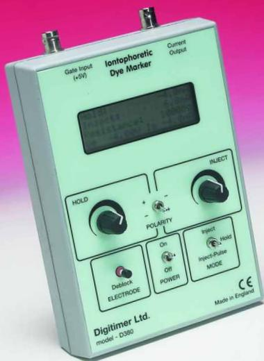
The D380 provides an isolated bipolar constant current output intended for the marking of individual neurons with dyes, such as Lucifer Yellow, via iontophoresis. Holding currents of up to  $\pm 6\text{nA}$  and injection currents up to  $\pm 12\text{nA}$  are provided and set by single turn panel mounted controls. These tactile controls permit use of the unit whilst using a microscope.
